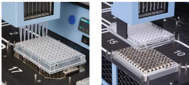
The ArrayPrep System automates reaction setup and magnetic bead purification of labeled products.
